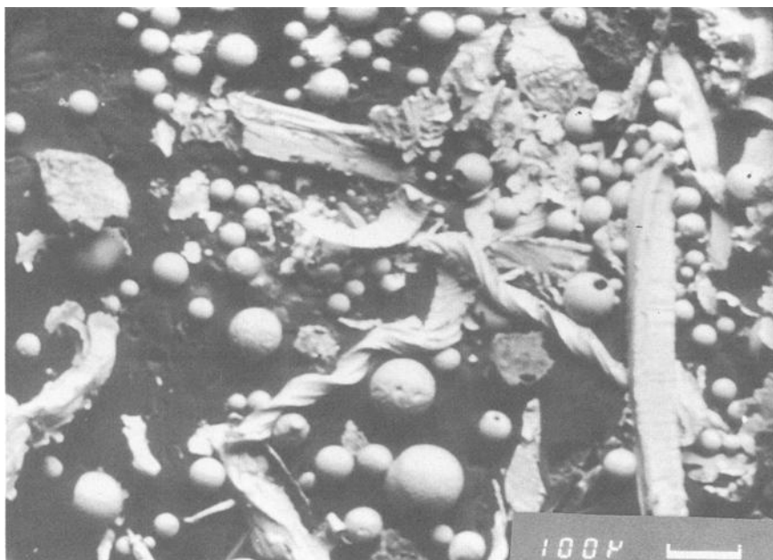
FIG. 4—SEM micrograph of particles from plain steel around cutting area.
